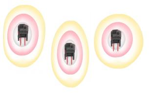
Operators should also be aware that one truck may sense the proximity of another more quickly—depending on direction of travel and size of the configured field—creating a slight difference in timing between alerts.
