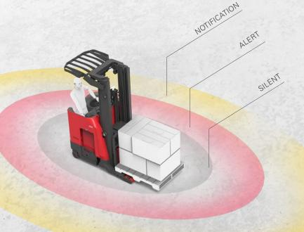
To optimize efficiency, each MFG zone size can be individually adjusted to suit a specific application or facility.
