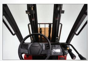
Open view mast provides the best line of sight for the task at hand.
